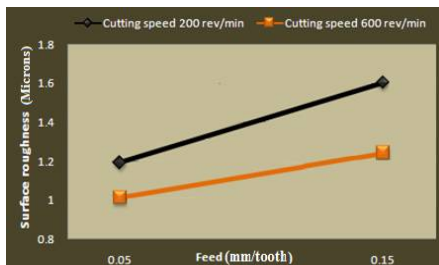
Fig.7: Interaction plot between cutting speed & feed for surface roughness
