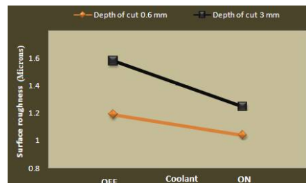
Fig.8 interaction plot between surface roughness and coolant
